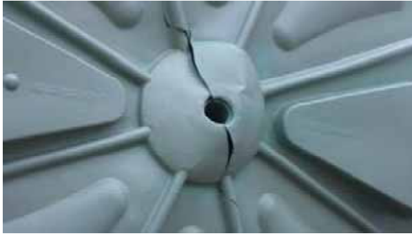
Existing Aqua tank with crack at the top of the tank.
